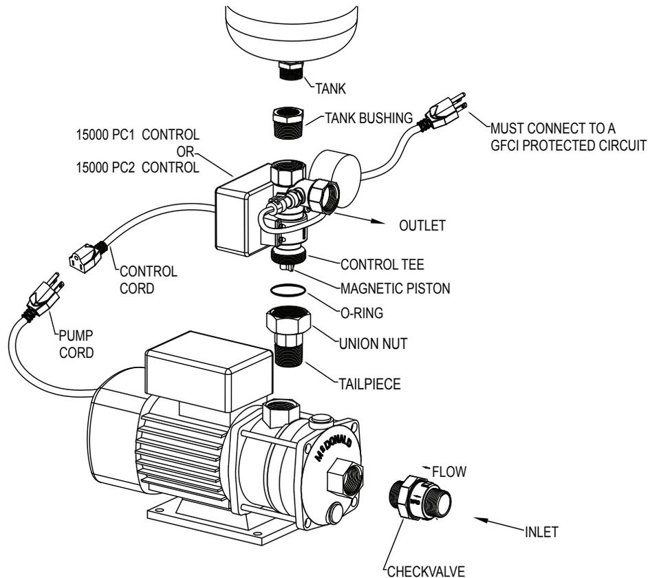
1. Apply pipe sealant on male threads of check valve. Thread into inlet of pump. **DO NOT apply any pipe sealant on pump threads.** Excessive pipe sealant or Teflon tape may foul check valves.
