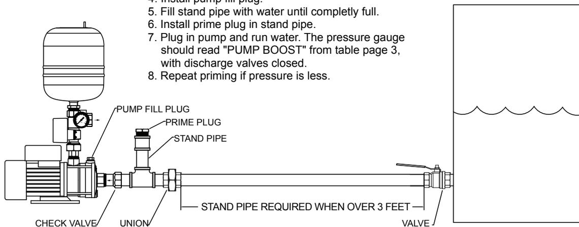
**Suction Lift** has the pump located higher than the level of the water. The DuraMAC™ booster can work in this application up to 10 feet, as long as the pump is fully primed. Air pockets and suction pipe leaks will cause the pump to accumulate air, and will eventually cause a Red light fault. However, if the pump inlet is the highest point, it is fully primed, a good check or foot valve is installed, a standpipe is installed, and there are no suction leaks, the pump will perform well.
